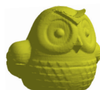
Scanning result of the rubber spray-coated object
